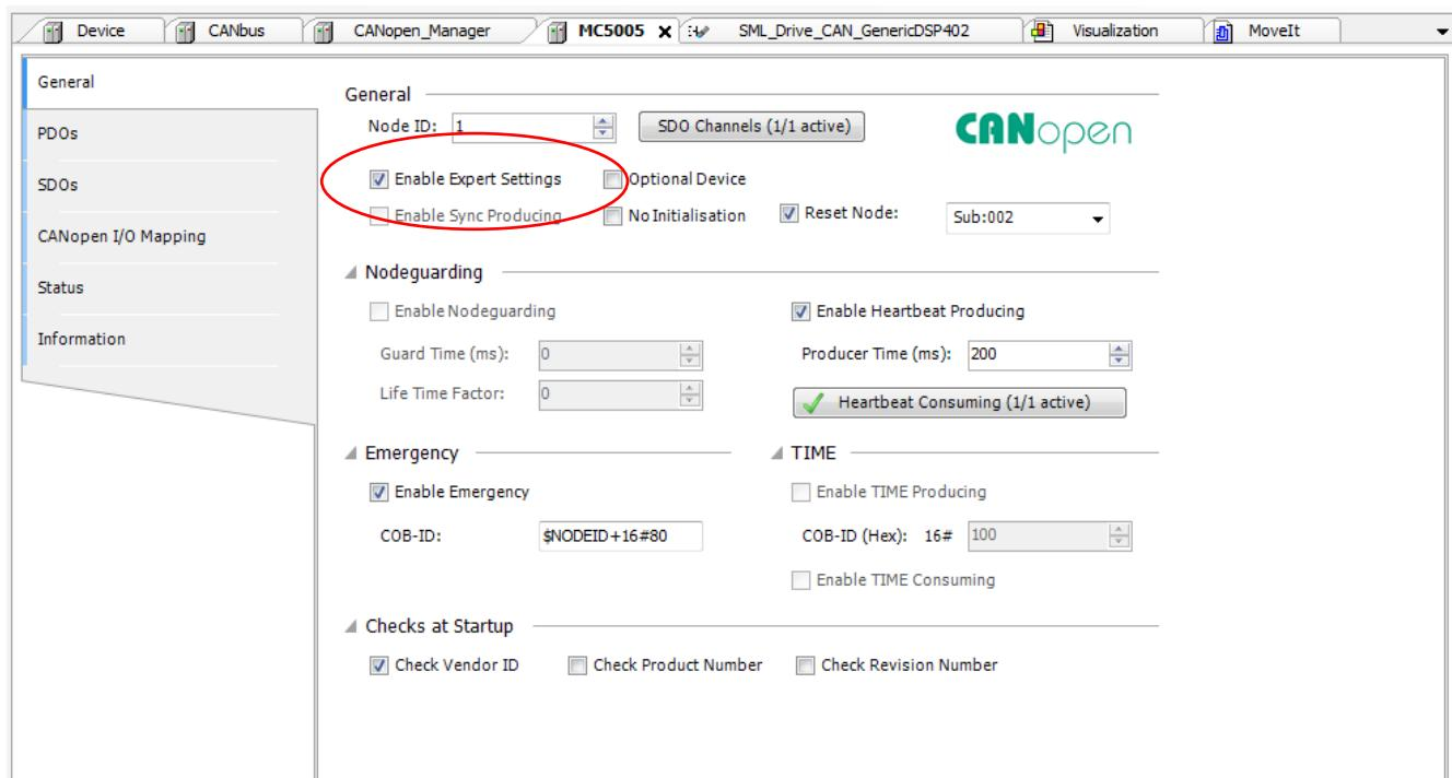
**Figure 7 General settings of the inserted CAN drive**
