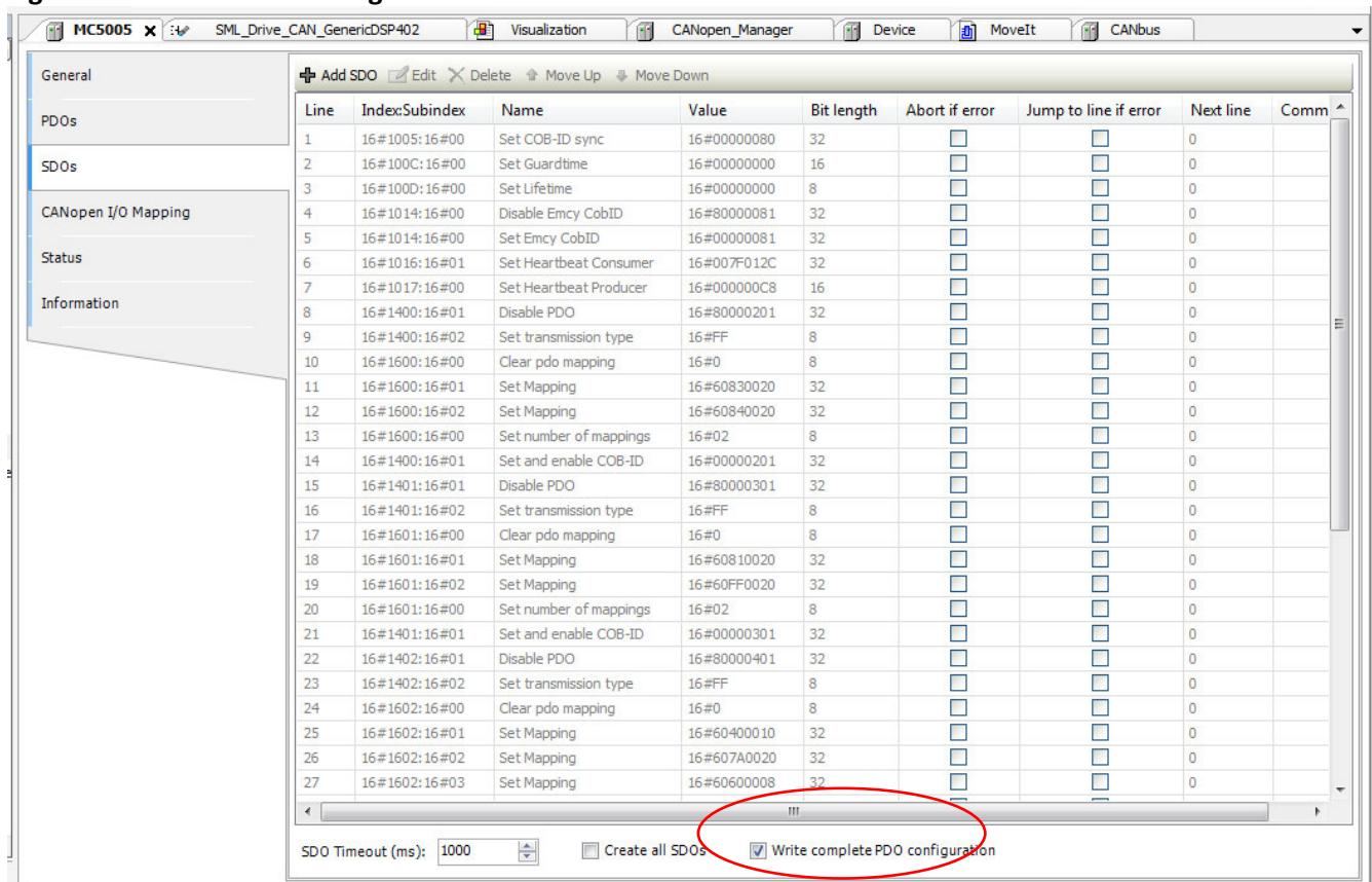
**Figure 14 SDO tab of the settings which lets you define which part of the drive configuration shall be updated at startup**
