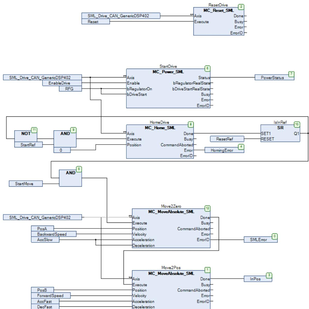
**Figure 17 Demo application using the SML FBs out of the library**
