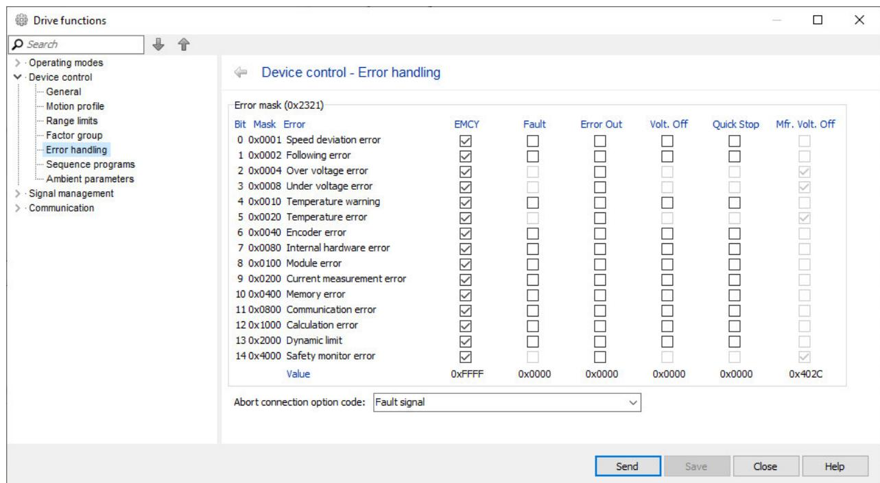
Figure 16 Configuration of the FAULT handling using the MotionManager
