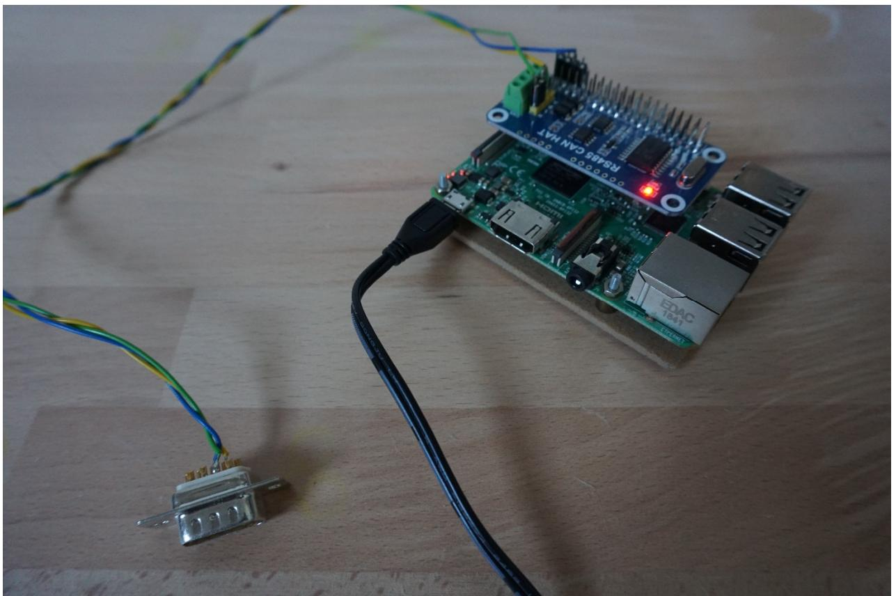
**Figure 1 RaspberryPi 3B equipped with the RS485 CAN HAT and a CAN cable**
