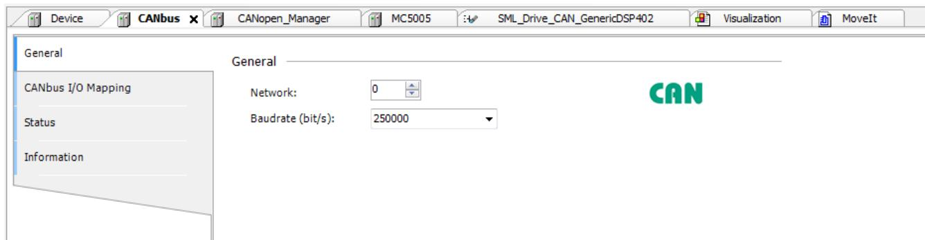
**Figure 2 CAN-bus specific settings**
