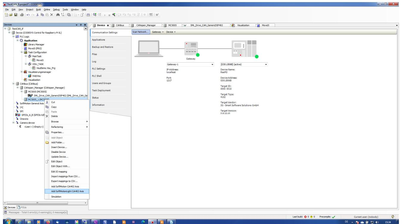
**Figure 8 Add a SoftMotionLight axis to the drive**
