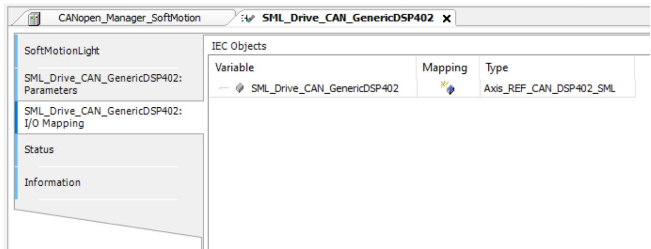
**Figure 15 Mapping of the SML axis - this object instance would be SML\_Drive\_CAN\_GenericDSP402**
