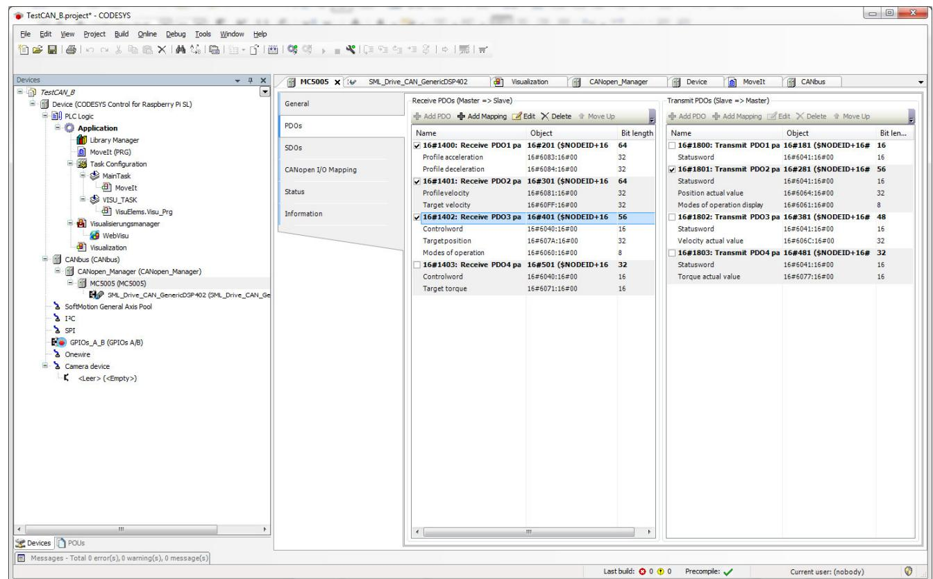
**Figure 12 PDO tab of the settings summarizing the PDO mappings**
