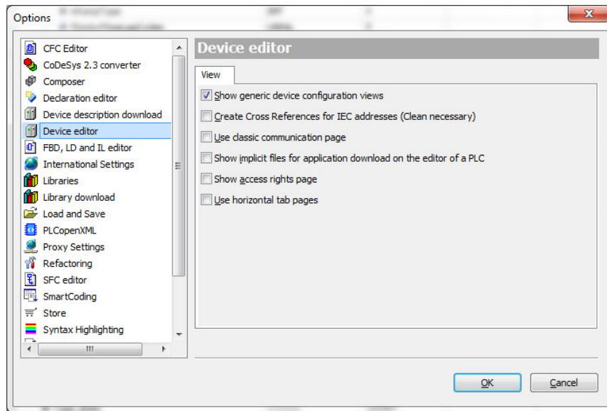
**Figure 9 Enable the generic device settings view for the Device editor**
