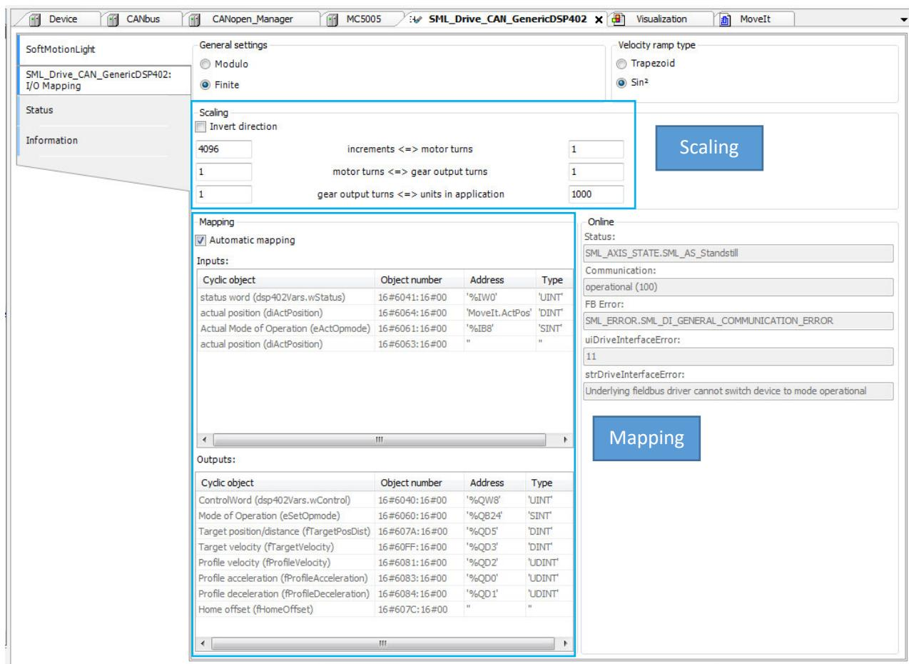
**Figure 11 Scalings and mappings of the axis**
