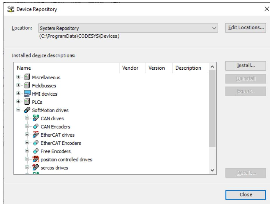
**Figure 5 CODESYS Device Repository window**
