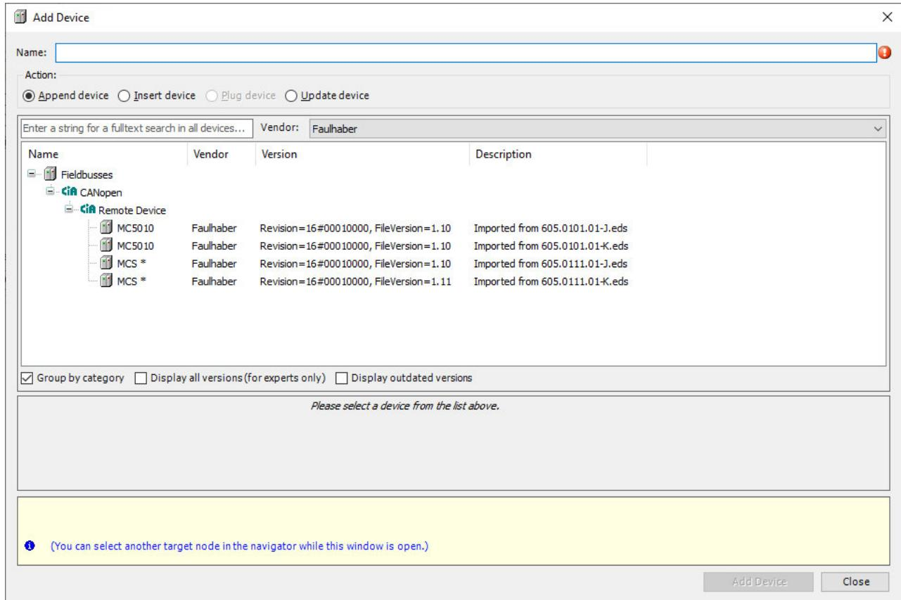
**Figure 6 Device Selection for the CAN-node to be added - here having a Filter to FAULHABER being the supplier**
