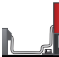
Figure 8: Routing close to the ground plane [1]
