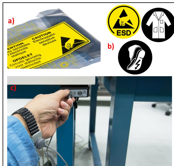
Figure 2: ESD-conform handling of encoders
