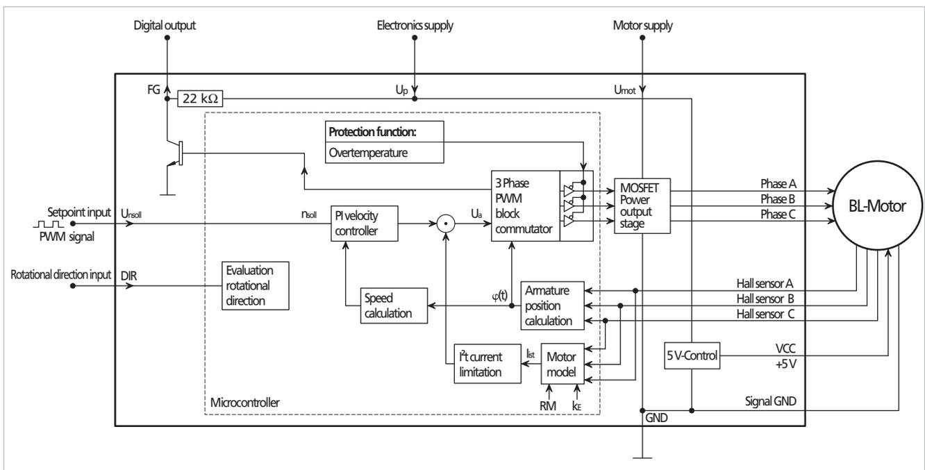
Fig. 35: Block diagram of a motor in PWM mode
