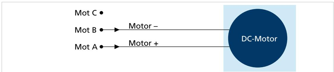
Fig. 11: DC motor without encoder (not SC 5004 and SC 5008)
