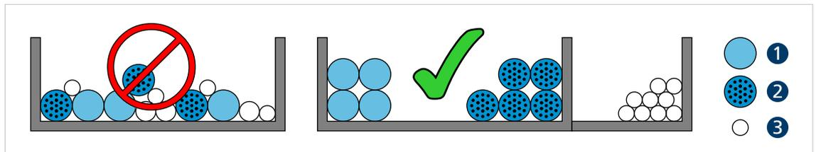
Fig. 18: Laying in the cable duct
