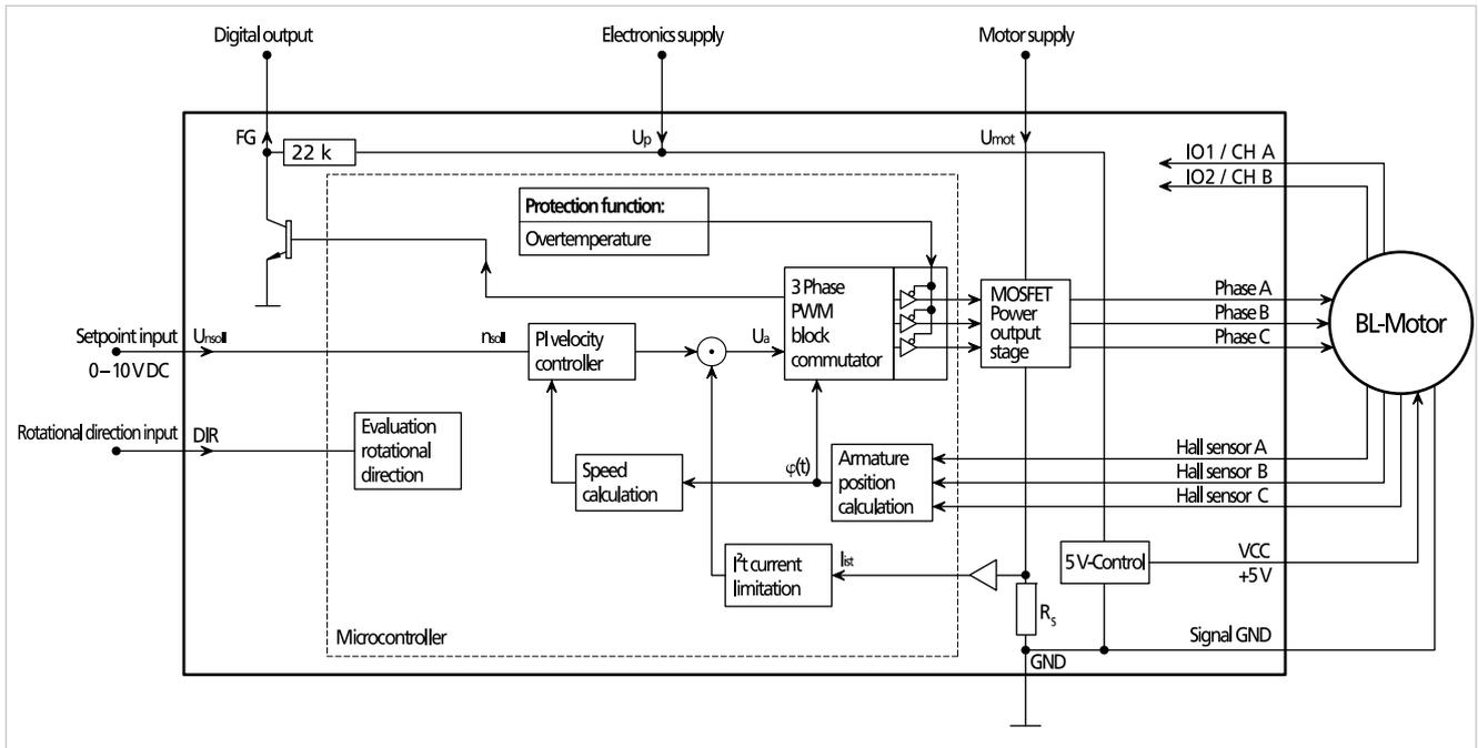
Fig. 33: Block diagram of a BL motor with digital Hall sensors and brake/enable
