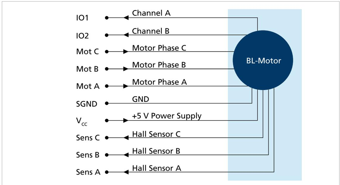
Fig. 16: BL motor with digital Hall sensors and incremental encoders (only option 4475)
