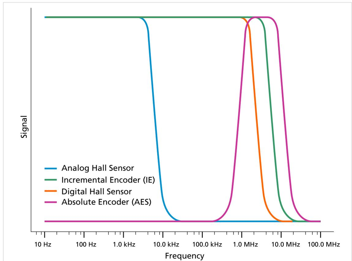
Fig. 23: Useful frequency ranges of the encoders
