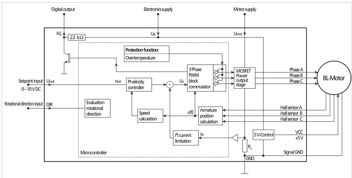
Fig. 29: Block diagram of a BL motor with analog Hall sensors
