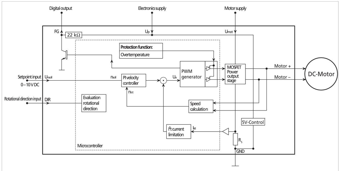
Fig. 27: Block diagram of a DC motor without encoder
