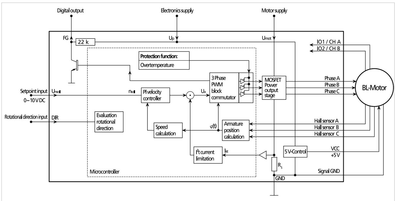
Fig. 32: Block diagram of a BL motor with digital Hall sensors and incremental encoders
