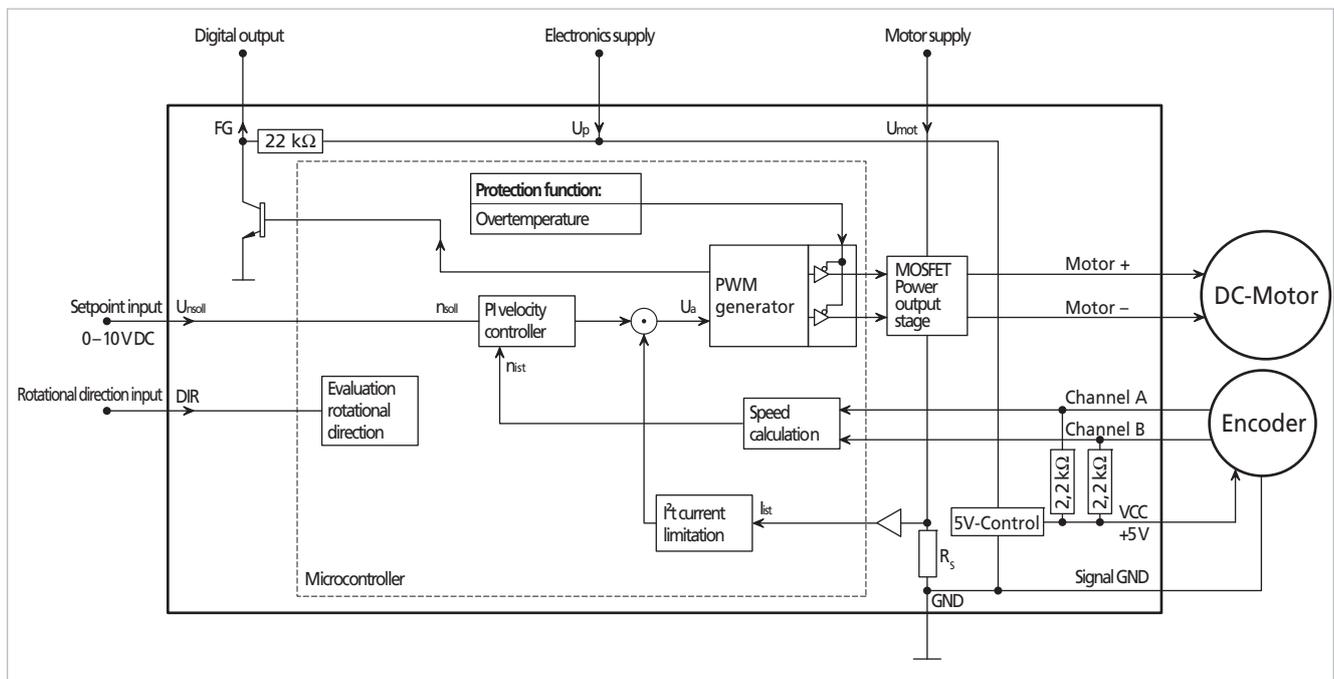
Fig. 26: Block diagram of a DC motors with encoder
