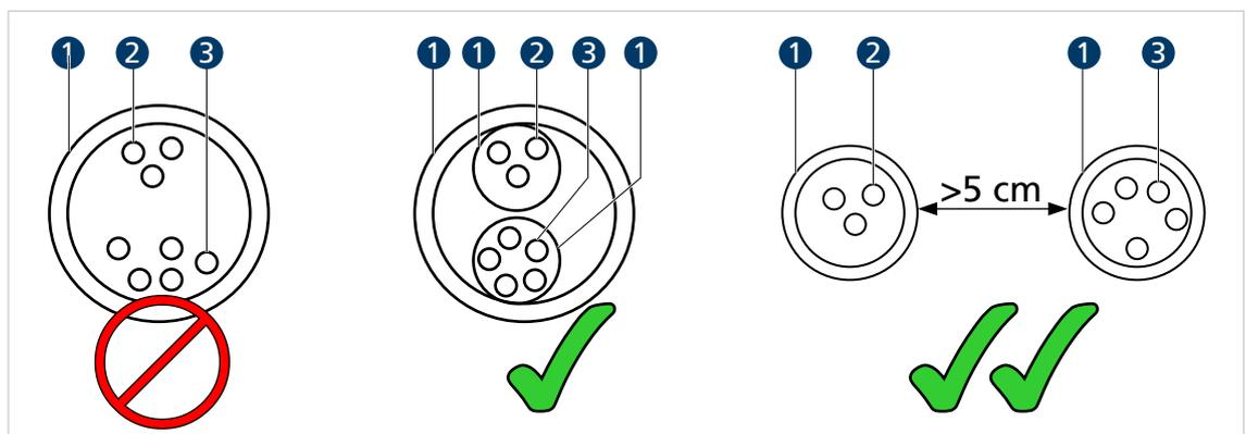
Fig. 19: Grouping and shielding of the cables
