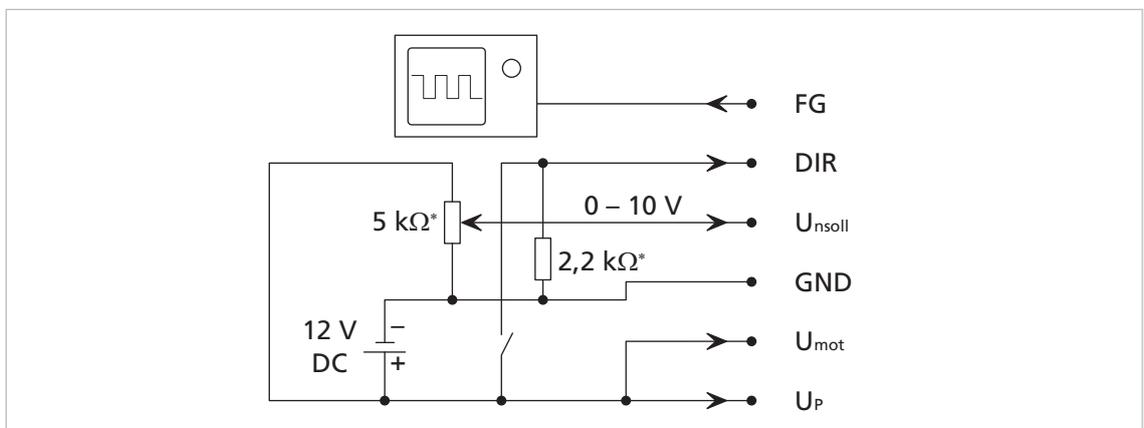
Fig. 9: Normal operation (speed set value specification by  $U_{nsoll}$ )
