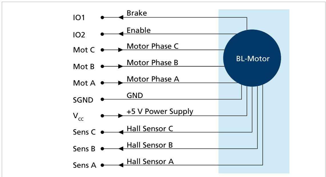
Fig. 17: BL motor with digital Hall sensors and brake/enable (only option 4476)
