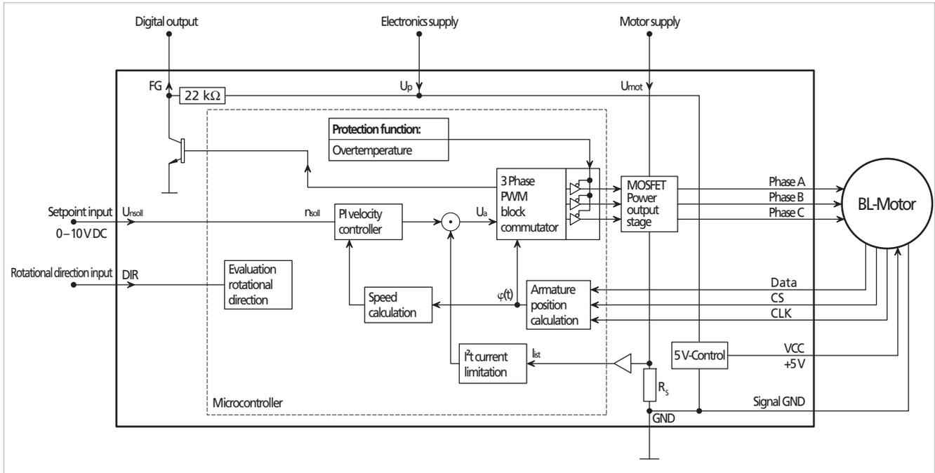
Fig. 31: Block diagram of a BL motor with absolute encoder
