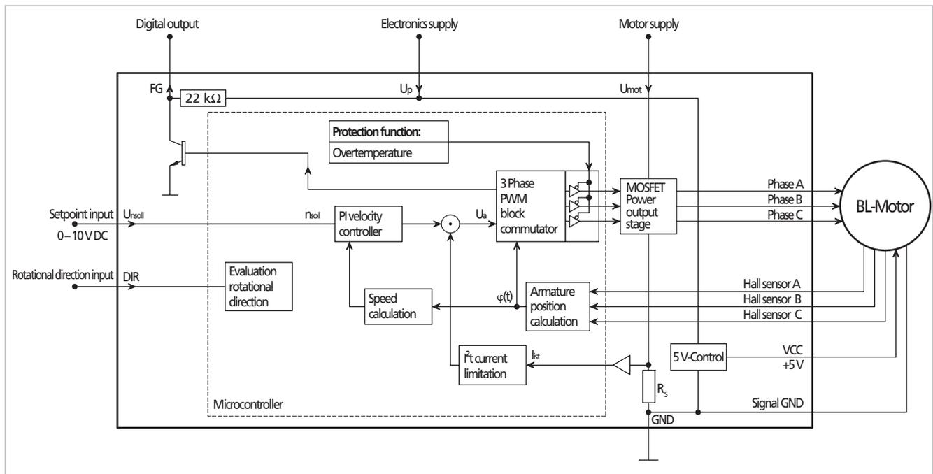
Fig. 28: Block diagram of a BL motor with digital Hall sensors
