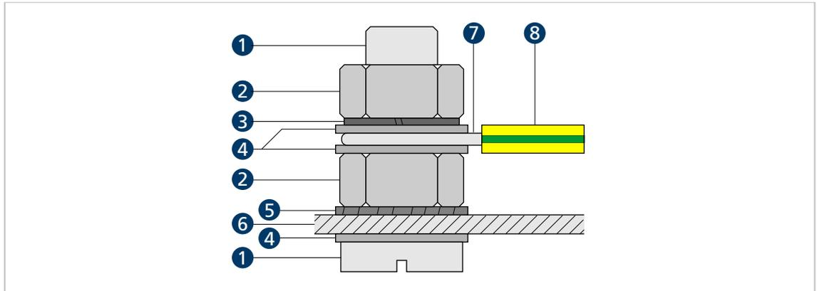
Fig. 22: Shield connection with cable lug
