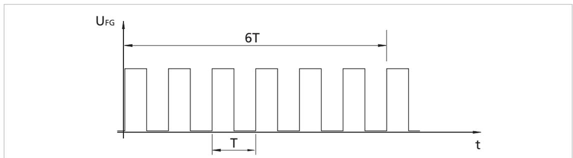
Fig. 36: Signal structure of frequency output
