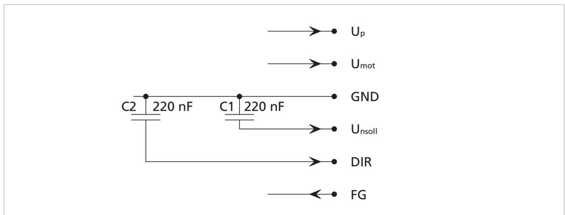
Fig. 4: EMC suppressor circuit with ceramic capacitors
