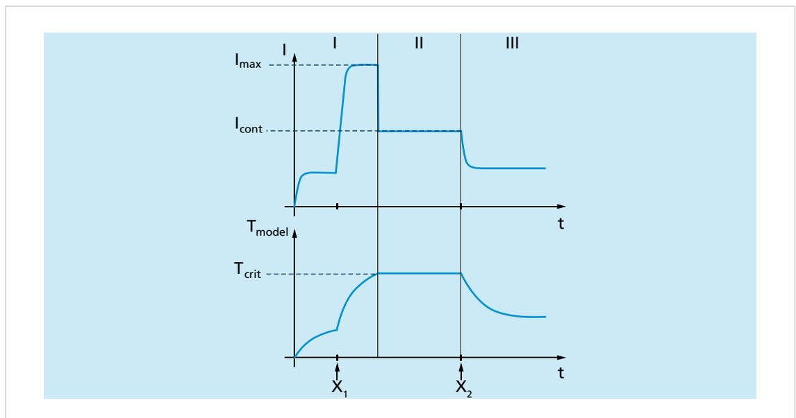
Fig. 38: Example of I<sup>2</sup>t current limitation
