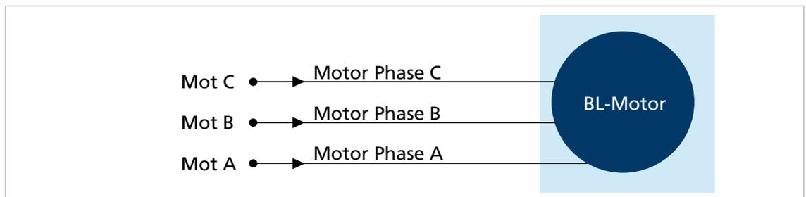
Fig. 13: BL motor without Hall sensors (not SC 5004 and SC 5008)
