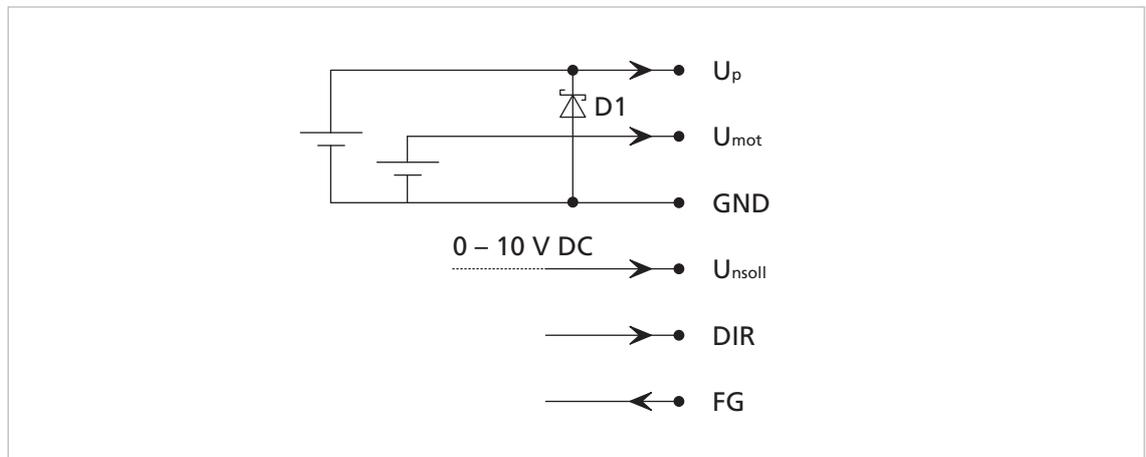
Fig. 6: EMC suppressor circuit for SC 2804 and SC 5008 with suppressor diodes
