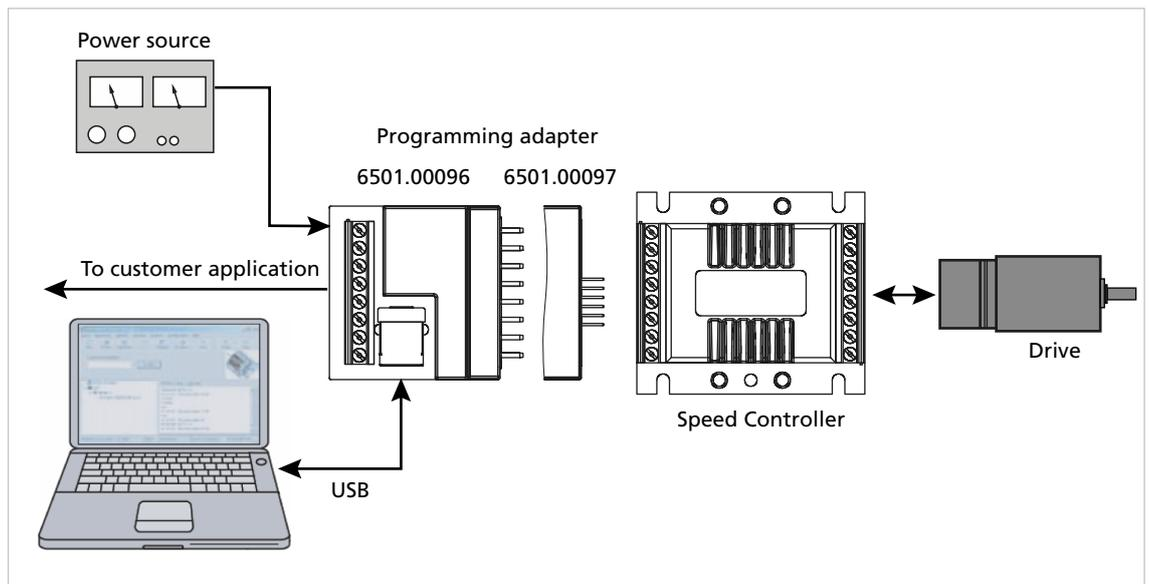
Fig. 41: Setup with programming adapter
