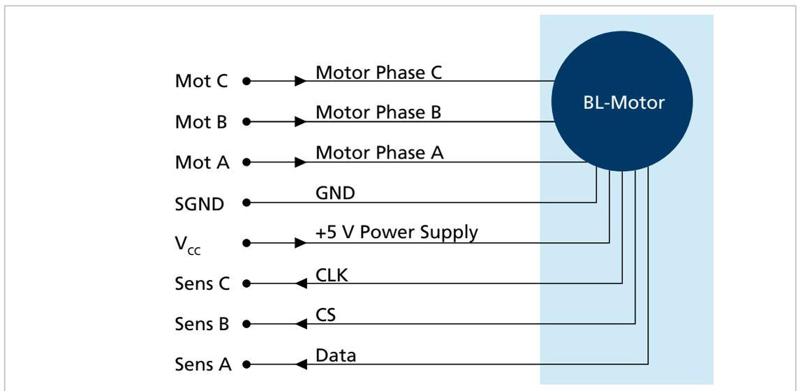
Fig. 15: BL motor with absolute encoders
