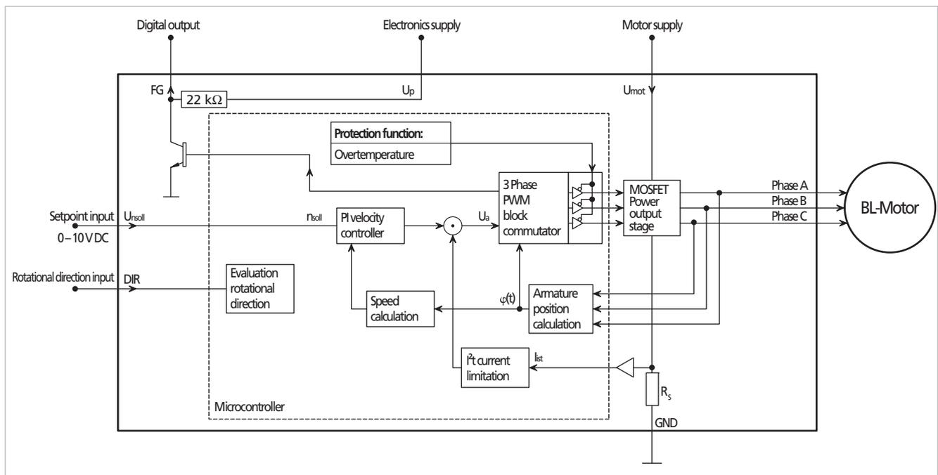
Fig. 30: Block diagram of a BL motor without Hall sensors
