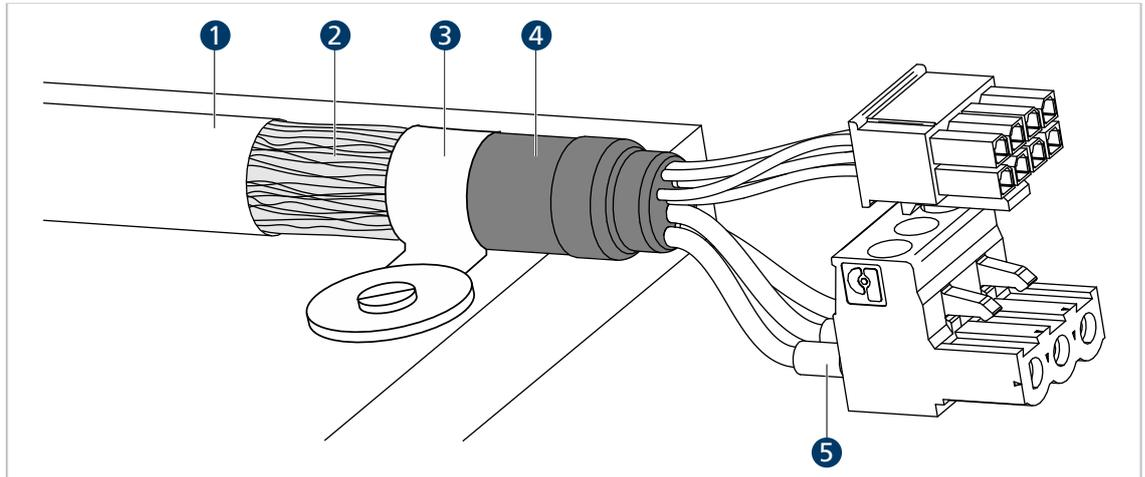
Fig. 21: Motor cable shield connection
