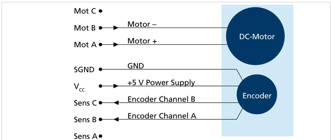
Fig. 12: DC motor with encoder
