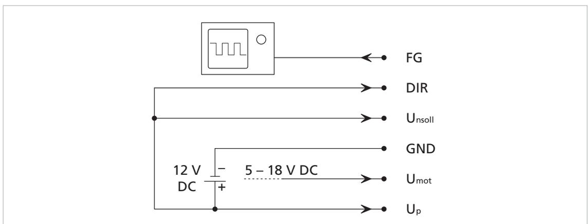
Fig. 10: Full modulation (motor speed is determined by  $U_{mot}$ )
