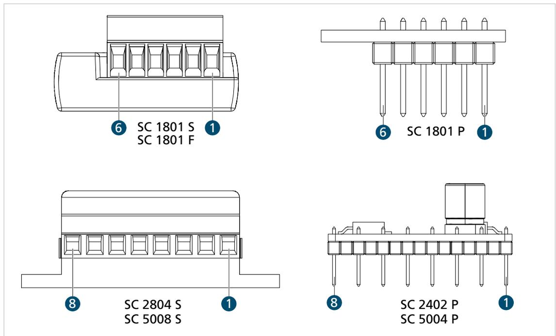
Fig. 7: Connections on the supply side
