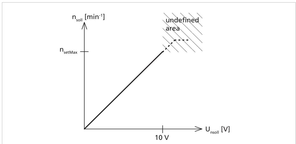
Fig. 34: Set value determination for Speed controller
