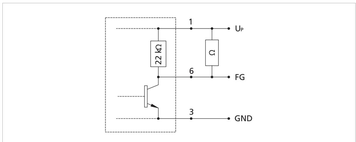
Fig. 37: Connection of an additional pull-up resistor
