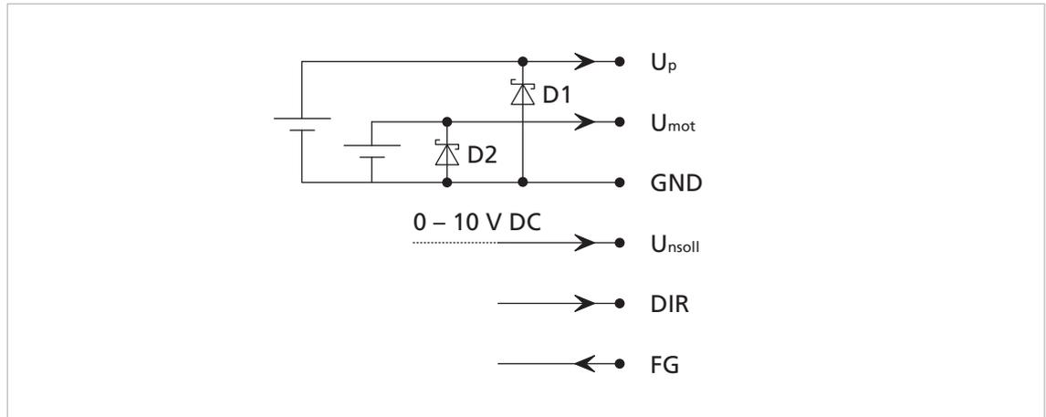
Fig. 5: EMC suppressor circuit for SC 1801 with suppressor diodes
