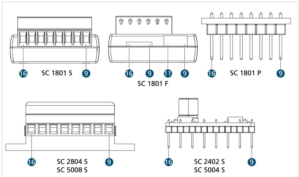
Fig. 8: Connections on the motor side
