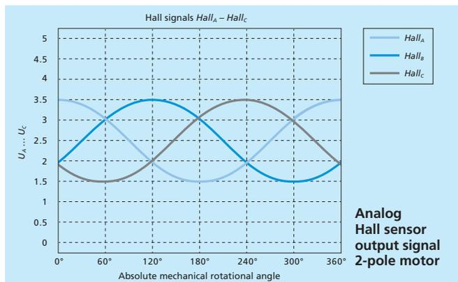
Due to the higher resolution, the analog Hall sensors can also be used for precise speed or position control, making them an especially economical, lightweight and compact alternative to encoders. The option for analog Hall sensors can be found directly in the data sheets of the motors
