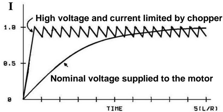
Figure 10 : Comparison of the current curve. [1]
