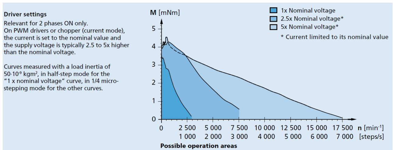
Figure 11 : Torque vs. speed curves for an AM1524 motor controlled by Trinamic TMC110 driver. The three curves correspond to three different driver supply voltage (i.e. 1x, 2.5x and 5x the motor nominal voltage).
