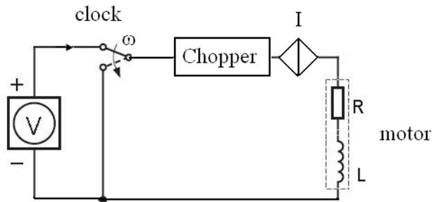
**Figure 9** : Schematic of a current mode system.
