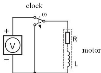
**Figure 3** : Schematic of motor driven at its nominal voltage.
