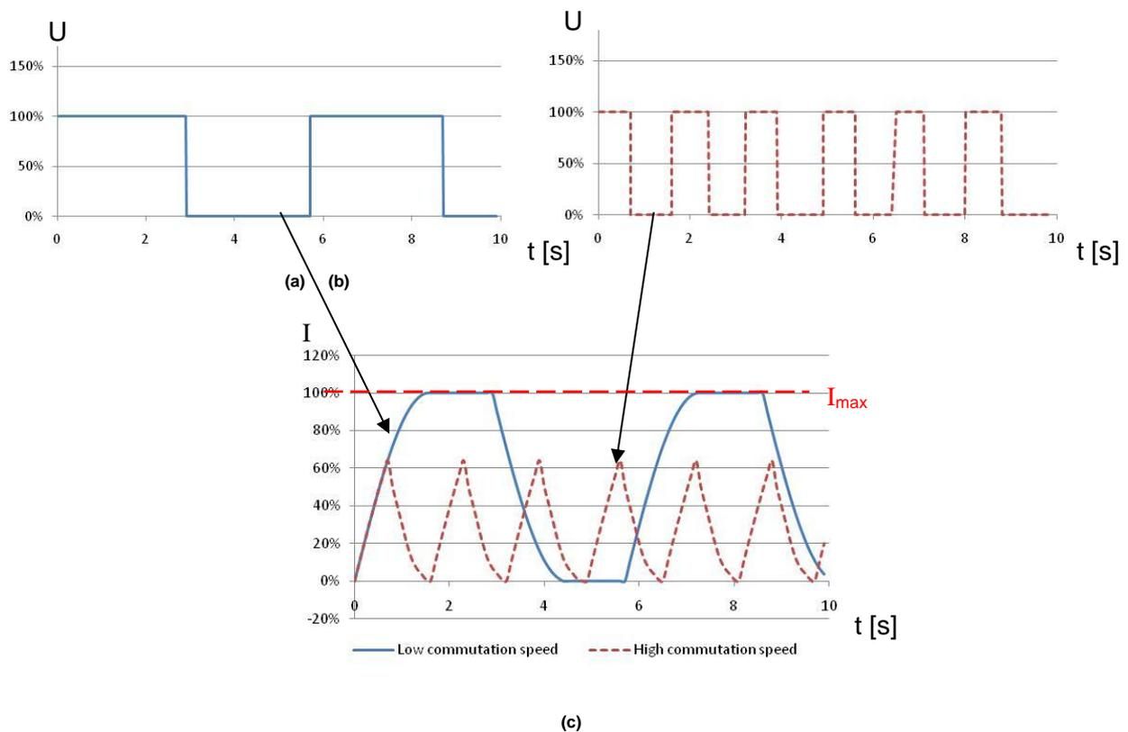
**Figure 4** : Voltage shape for a low (a) and high (b) commutation speed. The resulting current is plotted in (c).
