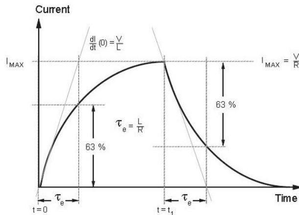
**Figure 2 :** Current in function of time. Current switched ON at  $t=0$  and switched OFF at  $t=t_1$ . Back EMF is set to 0; if this is not the case, the signal may have some oscillations due to the periodic back EMF shape.
