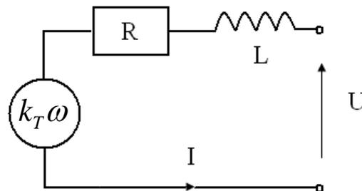
Figure 1 : Schematic design of a stepper motor.
