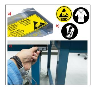
Figure 2: ESD-conform handling of encoders
